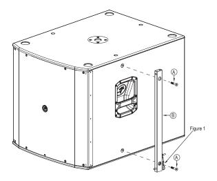
**Very important:** The bottom screw should be secure, but the locking pin should have the ability to be inserted through the holes in the tubing. With the pin inserted, tighten to the point JUST BEFORE pin movement is restricted. Do not over-tighten the screws, as this could damage the threaded inserts of the DRM18S subwoofer.
