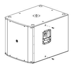
Align the pin side of the fly bar on the bottom of the DRM18S, with the handle side of the pin [Figure 1] towards the rear of the loudspeaker.
