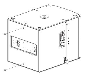
5. Apply Loctite 222 to the screws (C). Insert each screw through the flat washers (D), through the lock washers (E), then through the brace (F) into the two threaded inserts on the rear of the DRM18S, and securely tighten.
